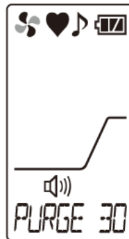
Automatic exhaust start (PURGE 30)
